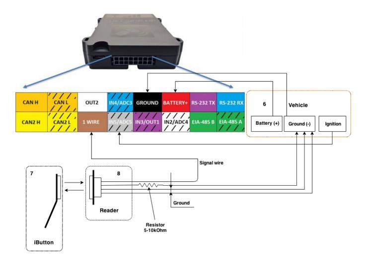
Note. Both ground wires should be twisted to a pair and connected to FM Blue device ground wire!
